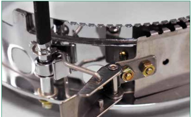
Latching Lever and Loop on hook
