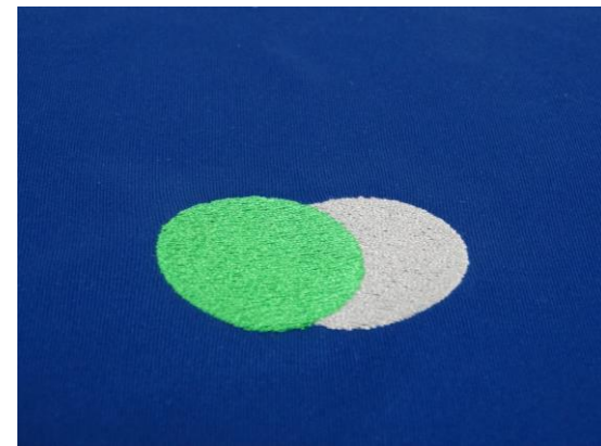
garment lays flat with proper digitizing technique
