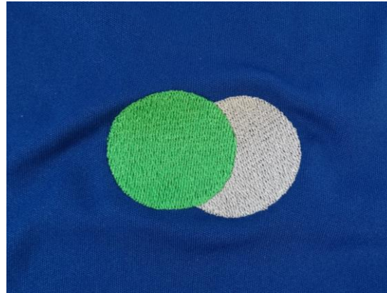
notice puckering and folding due to trapped fabric
