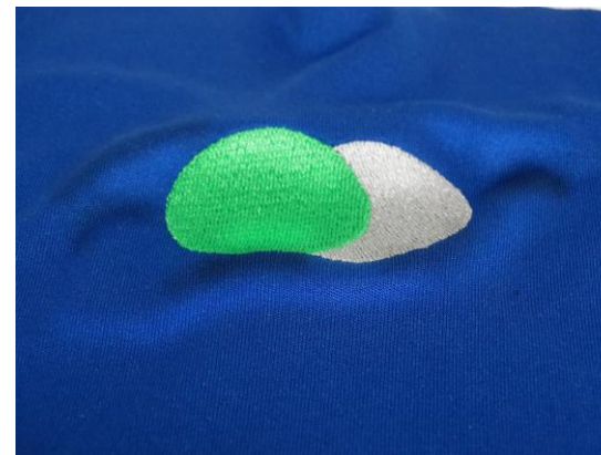
notice puckering and folding due to trapped fabric
